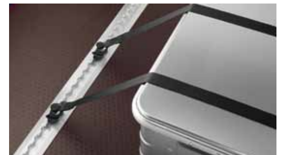
CARGO equipment package. The CARGO equipment package offers a high degree of flexibility for securing loads, thanks to a wooden floor with an integrated rail system, side wall lashing rails, straps and load-securing rings
