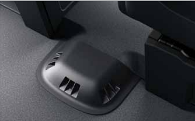
Heating / cooling air duct. The passenger compartment can also be brought to a pleasant temperature, thanks to a standard heating / cooling air duct leading to this area of the vehicle
